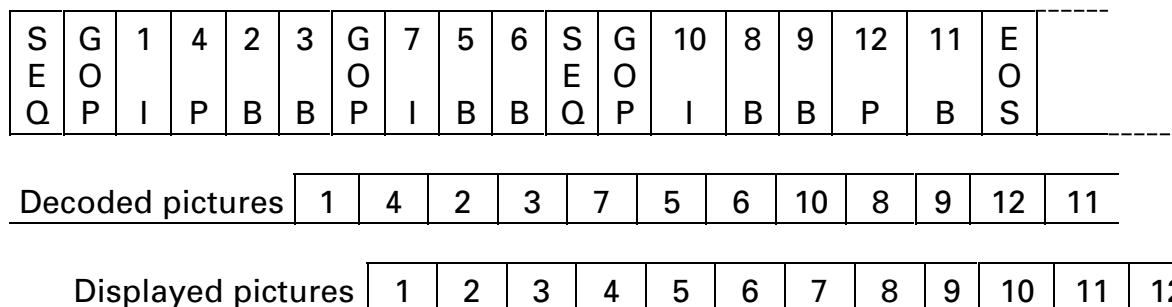
Figure IX.4.12 MPEG Video stream with decoded and displayed pictures
