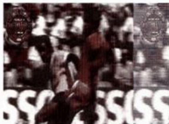
Poor CD-i MPEG encoding often results in blocky visuals. It's hardly a threat to VHS
