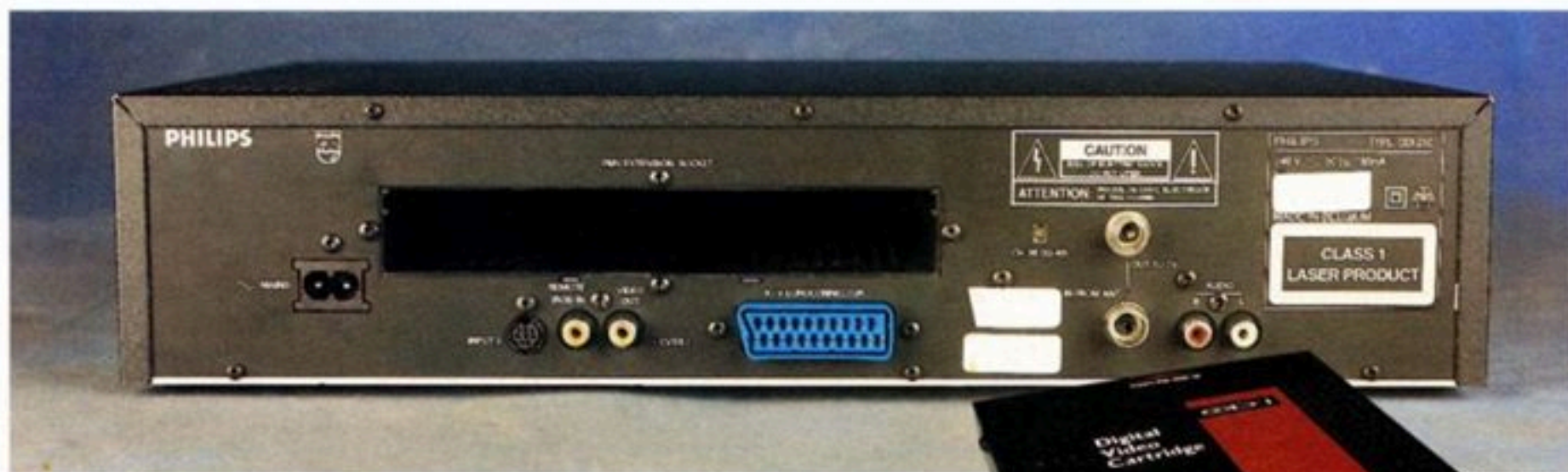
At the rear of the CD-i 210 are: a 21-pin SCART socket, audio and composite video RCA sockets, and the accommodating recess of the FMV port, for connection to the DV card
